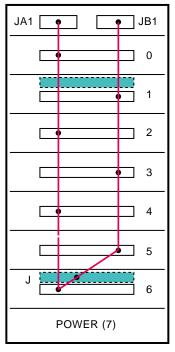
Figure 9-7: BA356 Internal SCSI Bus
